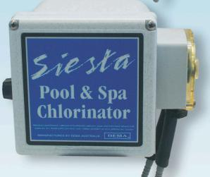
The SIESTA SEMI-AUTOMATIC CS-1P pool and spa chlorinator is an economical liquid chlorinator dosing unit that injects chlorine at regular intervals throughout the water filter cycle. It can also be used to inject set rates of acid at regular intervals to help maintain correct pH levels in pools or spas.
